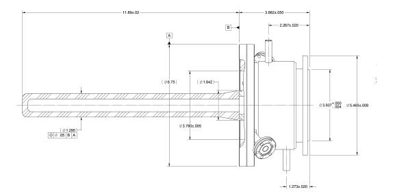
The VWP3143 Power Coupler was designed for ORNL's upgrade to the SNS system, as a higher power variant to the original VWP1133.
